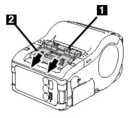
2. Push the black release lever down and toward the front of the printer to open the cover.
